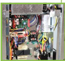
Digital Controls ensure proper operation, providing user-friendly diagnostics. Control box swings out for quick access to internal components.
