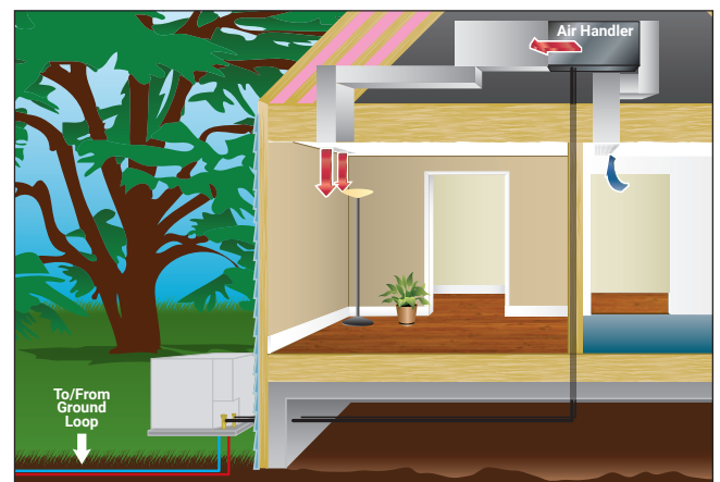
Common split geothermal installation with air handler.
