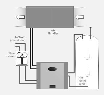
During the heating cycle, the fluid circulates through the loop extracting heat from the ground. The heat energy is transferred to the geothermal unit. The unit compresses the extracted heat to a high temperature and delivers it to your home through a normal duct system.
