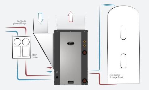
During the heating cycle, the fluid circulates through the loop extracting heat from the ground. The heat energy is transferred to the geothermal unit. The unit compresses the extracted heat to a high temperature and delivers it to your home through a normal duct system.
