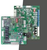
Aurora Advanced Controls, which offers two way communication between components, true energy monitoring, hot water generation control, IntelliZone2 zoning compatibility, and advanced troubleshooting capabilities. When paired with the Aurora WebLink (AWL), communication is enabled with the internet/smart grid and home automation networks. Optional Aurora Premium Controls adds Refrigeration and Performance monitoring, the most advanced diagnostics system in the industry.
