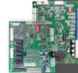
7. Aurora Controls: The powerful Aurora Base Control (ABC) offers two way communication between components, advanced operating logic and robust troubleshooting capabilities. The Aurora Expansion Board (AXB) adds support for true energy monitoring as well as compatibility with the Symphony Home Comfort Platform and our IntelliZone2 zoning system.
