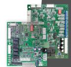
6. Aurora Premium Controls: The powerful Aurora controls offer two-way communication between components, operating logic, and robust troubleshooting capabilities. Diagnosis and setup are also simplified, making service much simpler for the technician.
