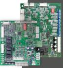
6. Aurora Controls: The powerful Aurora Controls offer two-way communication between components, advanced operating logic, and robust trouble shooting capabilities. Aurora also adds support for true energy and performance monitoring as well as compatibility with the Symphony Home Comfort Platform and our IntelliZone2 zoning system.
