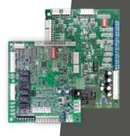
6. Aurora Advanced Controls: The powerful Aurora controls offer two-way communication between components, operating logic, and robust troubleshooting capabilities. Diagnosis and setup are also simplified, making service much simpler for the technician.
