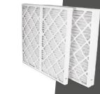
10. Filter and Filter Rack: Pleated MERV 11 filter is standard while an optional pleated MERV 13 is available for improved air quality. Filter rack holds 1" or 2" filters and is field convertible.
