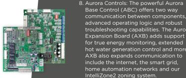
Base Control (ABC) offers two way communication between components, advanced operating logic and robust troubleshooting capabilities. The Aurora Expansion Board (AXB) adds support for true energy monitoring, extended hot water generation control and more. AXB also expands communication to include the internet, the smart grid, home automation networks and our IntelliZone2 zoning system.
