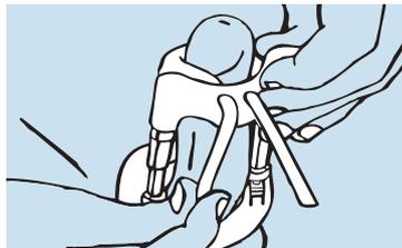
Finally, fit the ends of the silicone band into the grooves behind the upper plastic support carefully. You have to stretch the band while pressing into the grooves.
