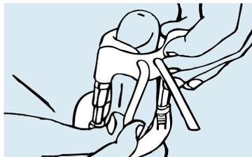
Finally, fit the ends of the silicone band into the grooves behind the upper plastic support carefully. You have to stretch the band while pressing into the grooves.
