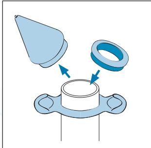
Remove the cone of the cylinder. Snap rings in place and place in the selected cushioning rings after applying Gel Lubricant.
