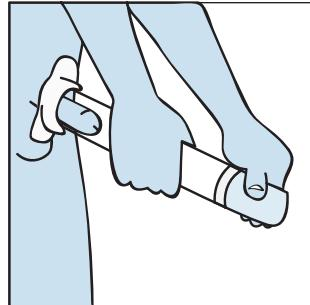
On the other end of the cylinder, snap in the electric motor, when fitted correctly there will be no movement and there will be a perfect seal.
