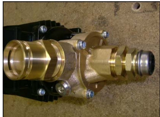
Figure 34 - Non Return Valve Fitting Location On Pump
