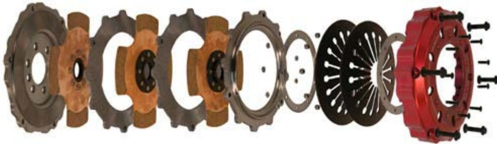
**Breakaway view of the 7.25 clutch assembly**
