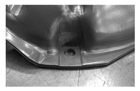
10.95 Borg & Beck clutches require a small head pressure plate bolt to avoid contact between the bolt head and the clutch disc through the bolt hole windows. Use bolt set 490 to correct this issue.
