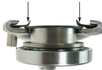
Incorrect installation - clips around rear of bearing
