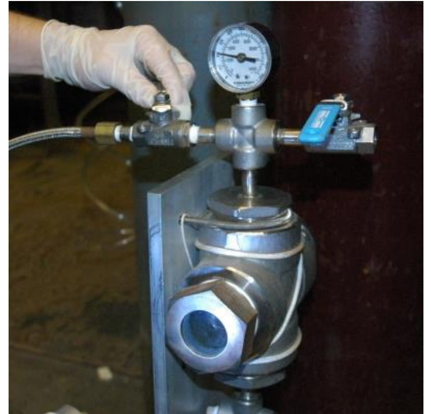
Conventional supercritical drying chamber
