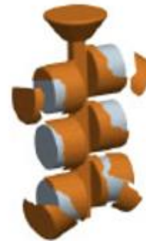
Removing Ceramic Mold
