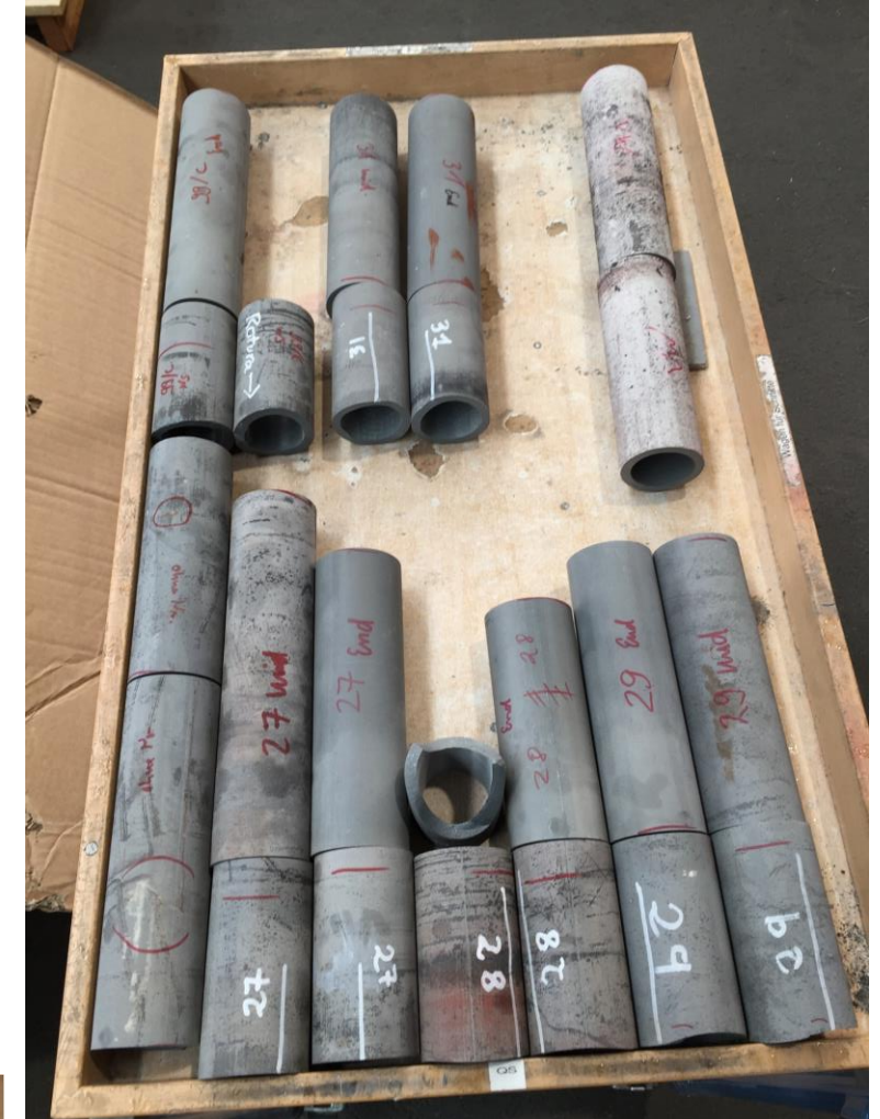
Pieces of rollers used in a large kiln - new rollers are 3 m long
