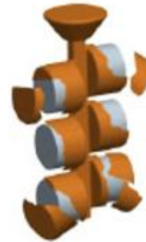
Removing Ceramic Mold
