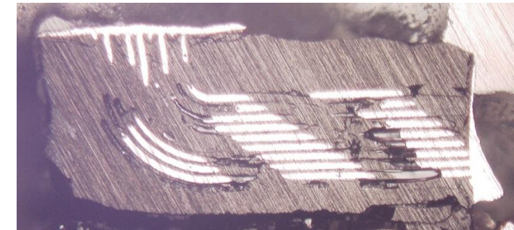
Cross-section after metallization (polishing off-axis to vias)
