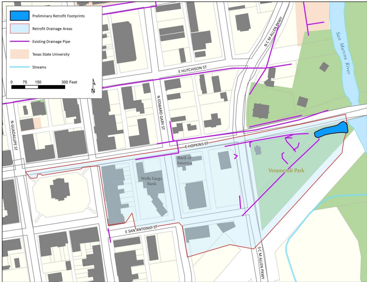
Figure 8-27 Hopkins Drainage Channel Pond 2 Retrofit: Concept Plan
