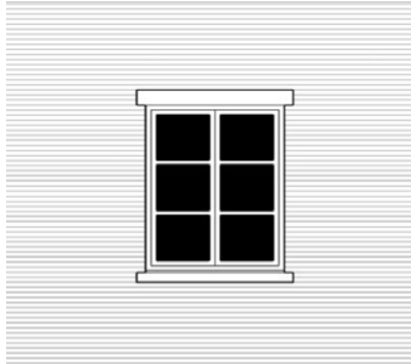
Lintels above windows should be expressed, especially in exposed masonry construction. Window sills must be expressed on the facade and shall protrude beyond the plane of the facade so as to form a drip edge.
