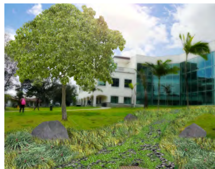
Proposed condition - Rain bioswale
