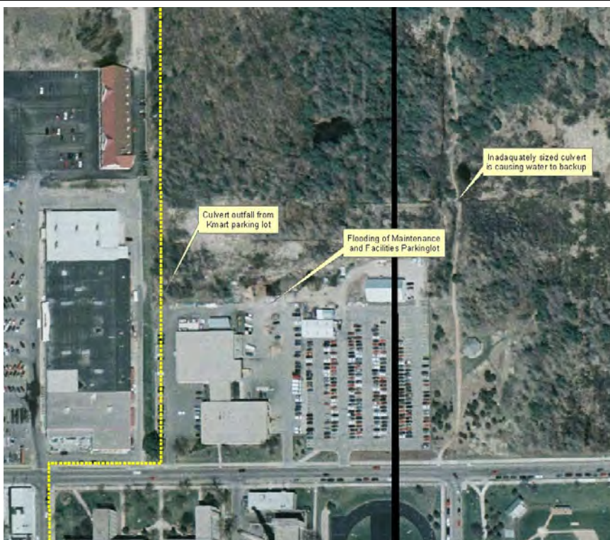
Figure 3-13 - Existing drainage problems
