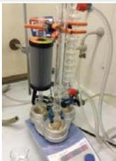
**Green Labs** In an effort to reduce water use in labs, Green Labs works with researchers to replace equipment with water-less versions, or more efficient pieces. Waterless, findensers eliminate the need for water entirely.
