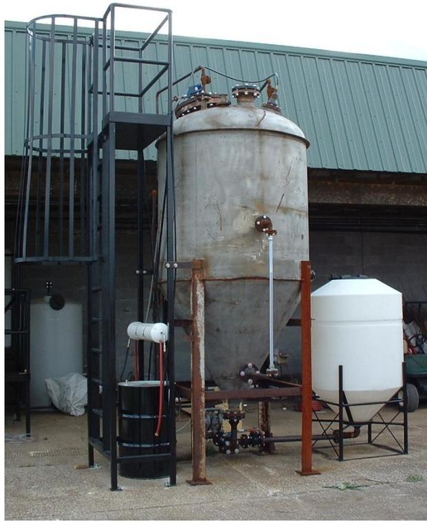
Figure 3: Main Reactor Vessel and Glycerin Processing Equipment
