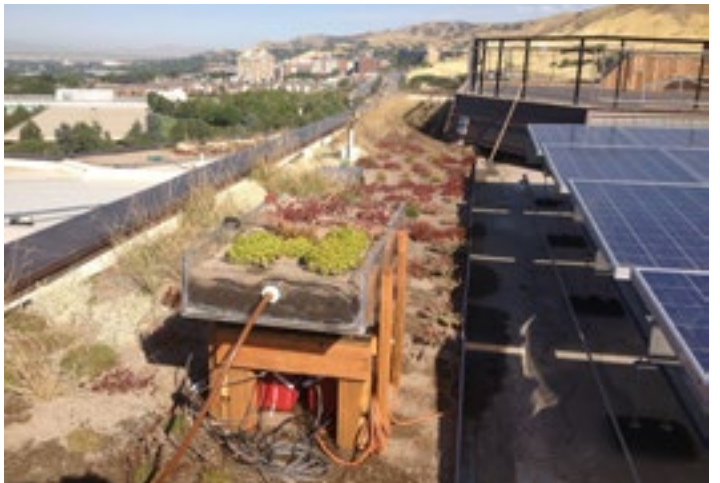
Green roof weighing lysimeter on the roof garden of Natural History Museum of Utah (Youcan Feng)
