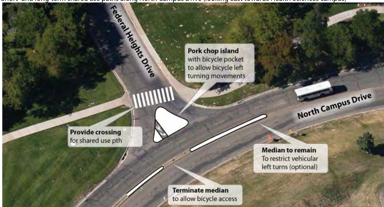
Conceptual strategy to allow bicycle left turns from Federal Heights Drive to North Campus Drive
