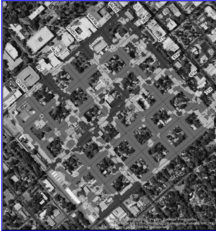
Figure 3. Students in the advanced Geographic Information Systems course used GPS and luminescence meters to measure actual street lighting levels along the sidewalks at over 2,000 locations along the South Campus Neighborhood's 42-square blocks. They then produced maps, such as this one, using ArcGIS, showing the variance in lighting levels at night across the neighborhood.
