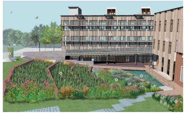
Sidwell Middle School recycles both grey water and stormwater. This LEED Platinum building also has passive heating and cooling systems. The wastewater treatment ponds provide many opportunities for exploration and explanation of water flow and biotic filtration.
