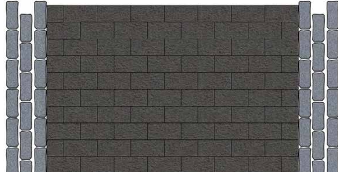
Triple Soldier Course Jumbo Blocks 6.5-12" x 6" Asphalt-Block Pavers Running Bond Triple Soldier Course Jumbo Blocks
