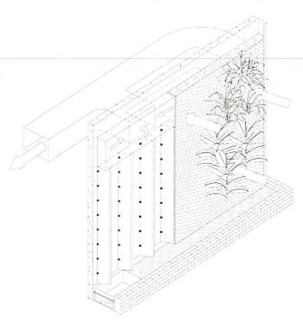
The biofilter is an adaptation of two industrial processes. The first being biofiltration which is the passing of contaminated air stream through a biologically active substrate where beneficial microbes use the pollutants (such as VOCs) as a food source. The second is phytoremediation; where green plants help the growth of these beneficial microbes.
