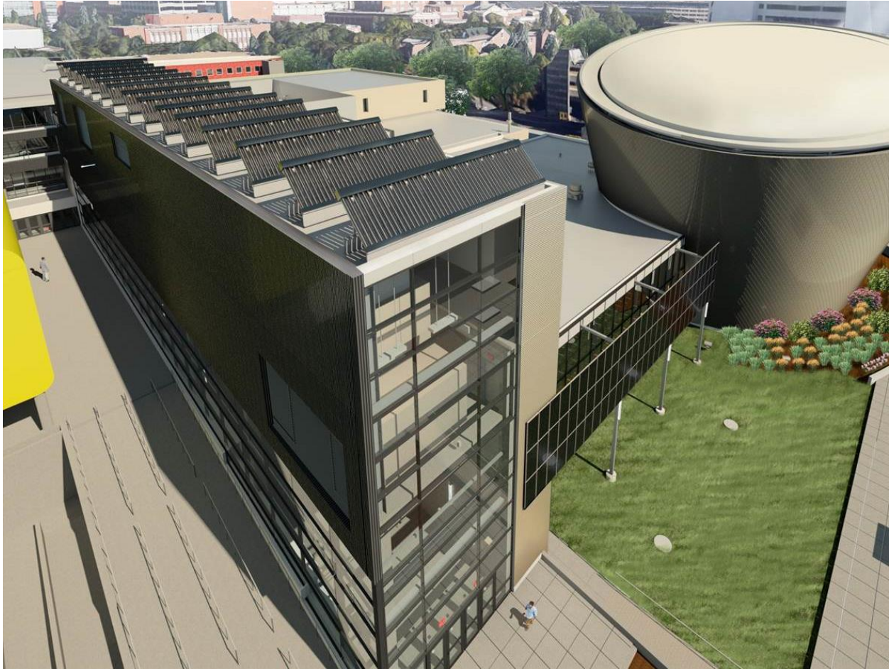
Figure 5. Artistic rendering of the PAW Centre, with solar thermal (top left) and solar PV (solar shade), courtesy of Group 2 Architecture.
