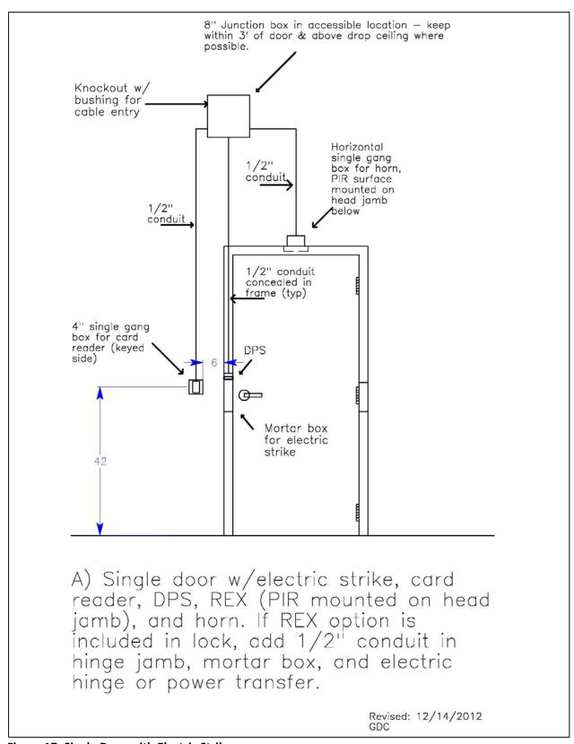
Figure 17: Single Door with Electric Strike
