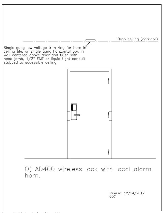
Figure 31: Wireless Lock with Local Alarm
