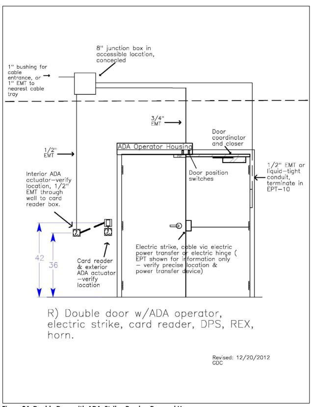
Figure 34: Double Door with ADA, Strike, Reader, Rex, and Horn
