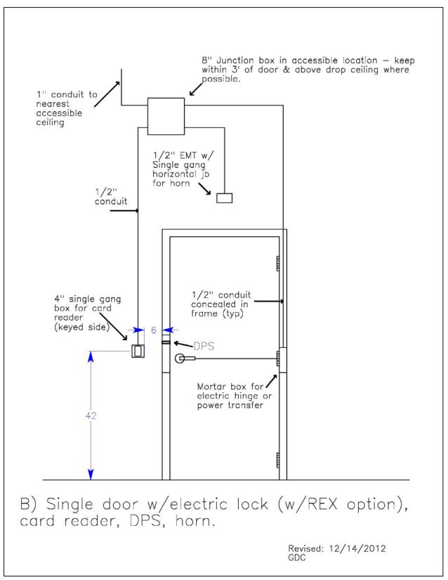
Figure 18: Single Door with Electric Lock
