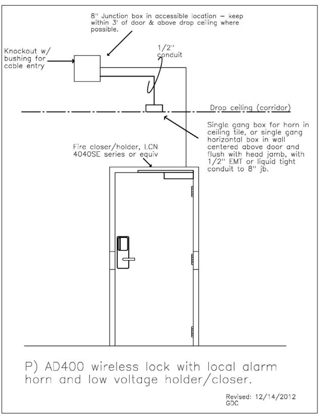
Figure 32: Wireless Lock with Horn, Holder, and Closer
