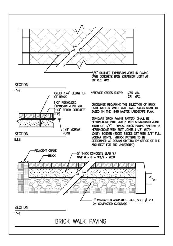
Figure 10: Brick Walk Paving
