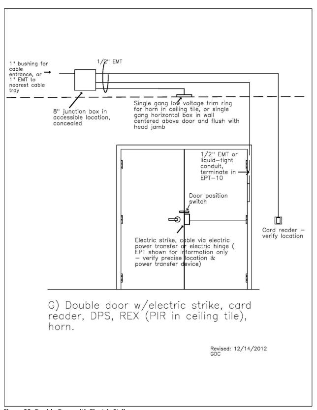
Figure 23: Double Door with Electric Strike
