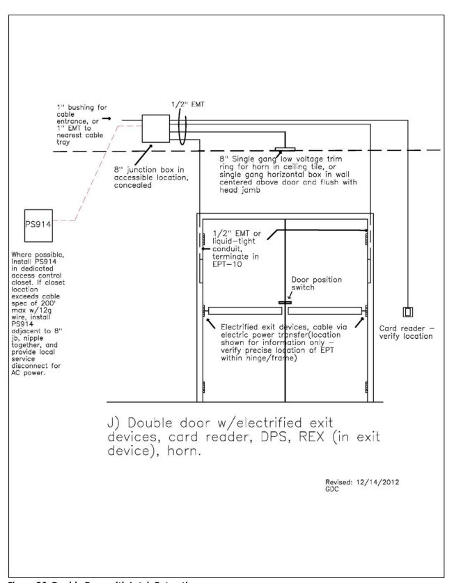
**Figure 26: Double Door with Latch Retraction**
