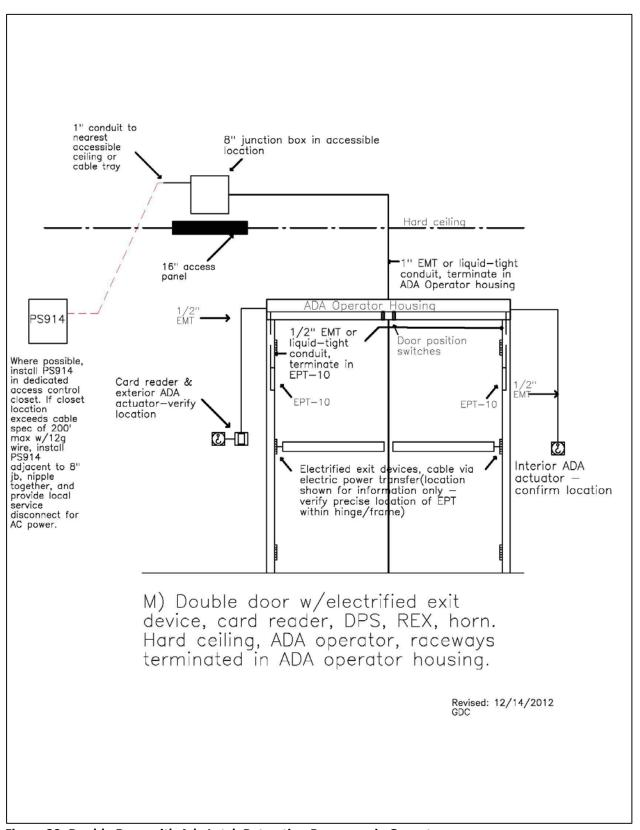
Figure 29: Double Door with Ada Latch Retraction Raceway via Operator
