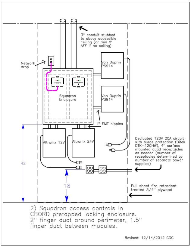
Figure 16: Squadron Controls in Enclosure
