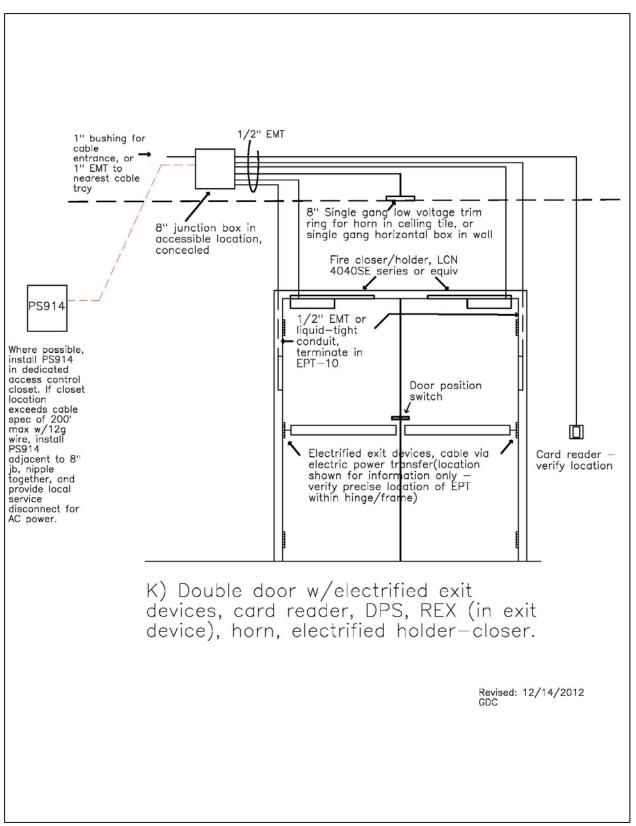
Figure 27: Double Door with Latch Retraction Holder
