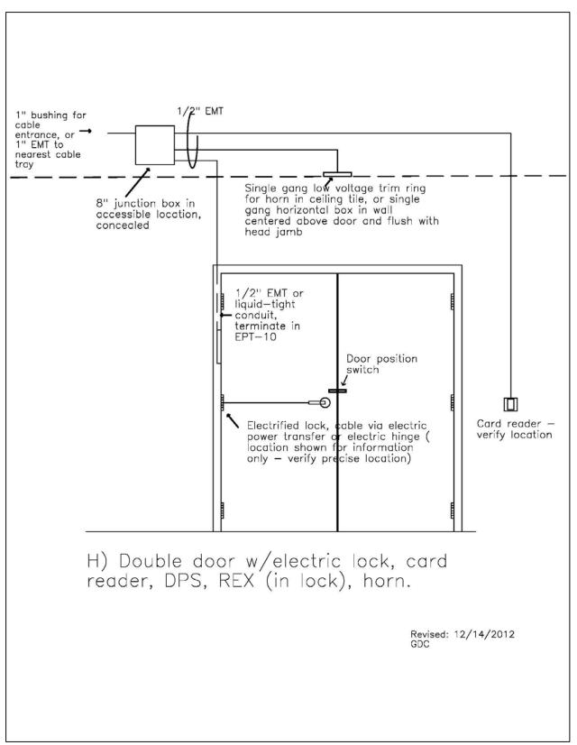
Figure 24: Double Door with Electric Lock
