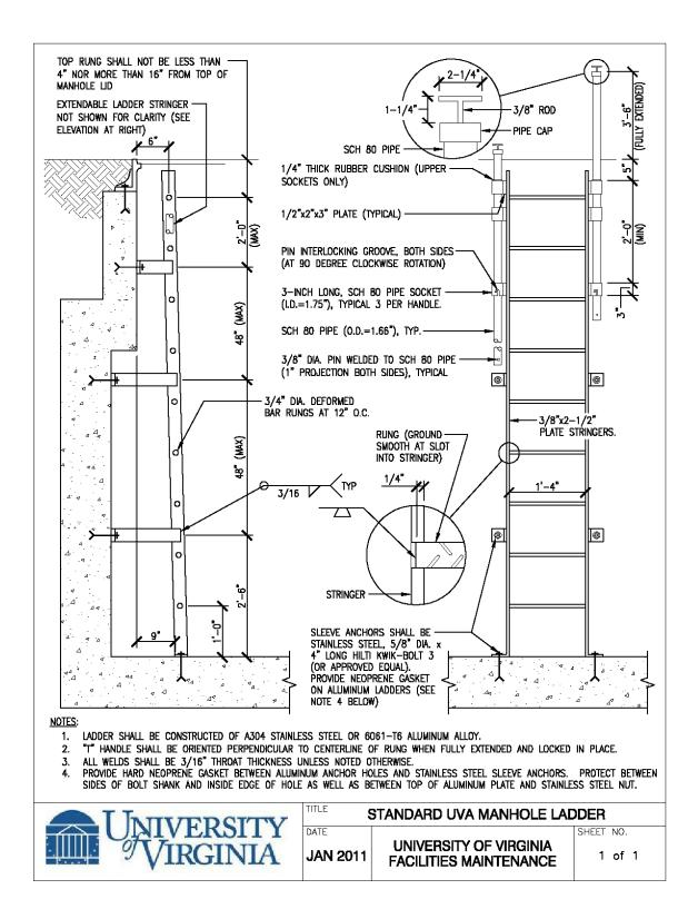
Figure 13: Standard UVa Manhole Ladder
