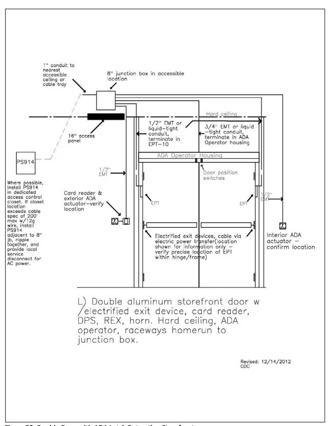
Figure 28: Double Door with ADA Latch Retraction Storefront
