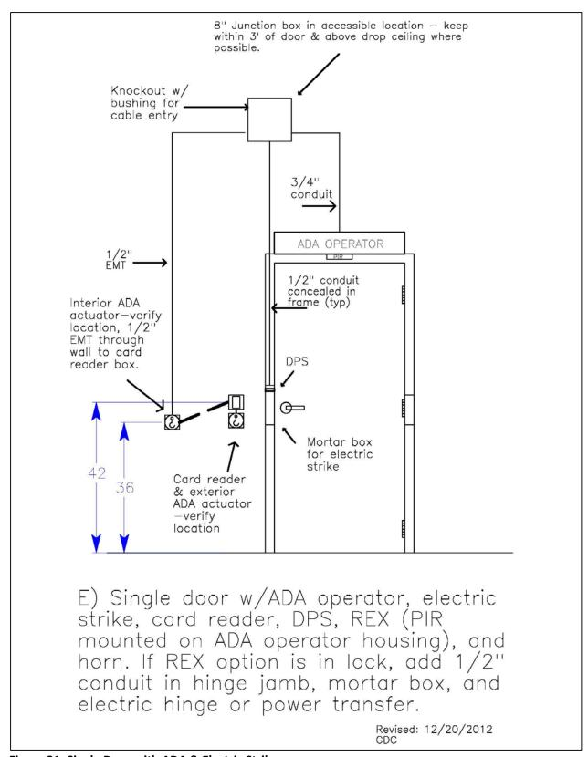
Figure 21: Single Door with ADA & Electric Strike
