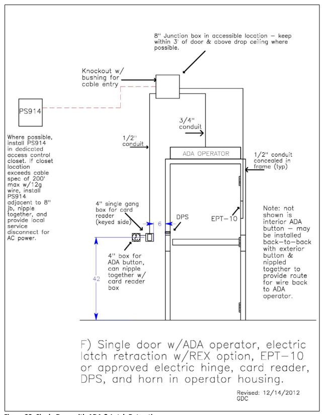
Figure 22: Single Door with ADA & Latch Retraction
