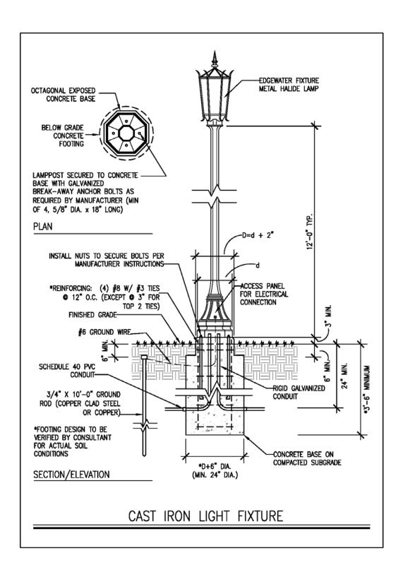
**Figure 6: Cast Iron Light Fixture**
