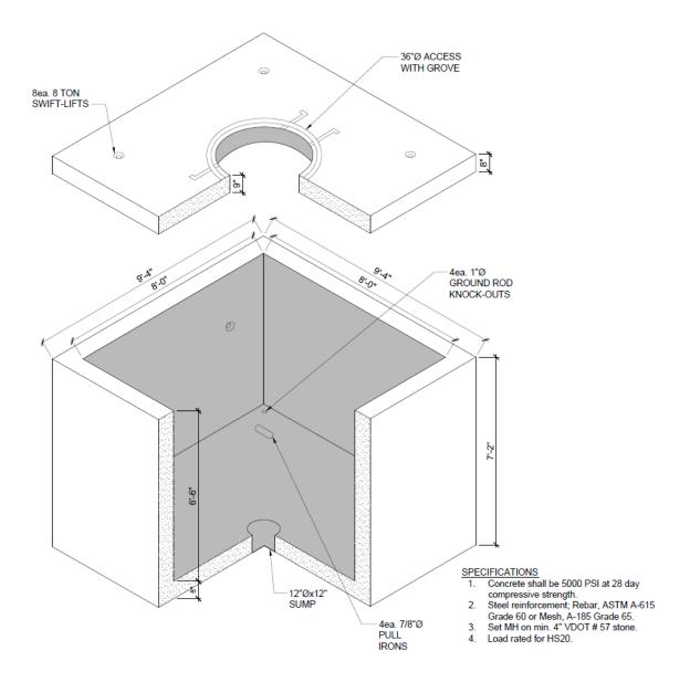
Figure 15: Electrical Manhole/Vault Detail
