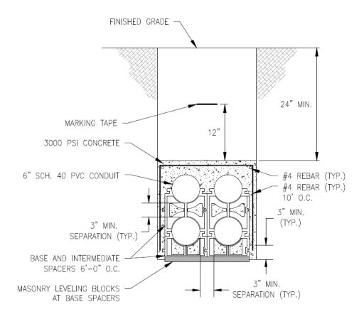
Figure 16: Electrical Ductbank Section
