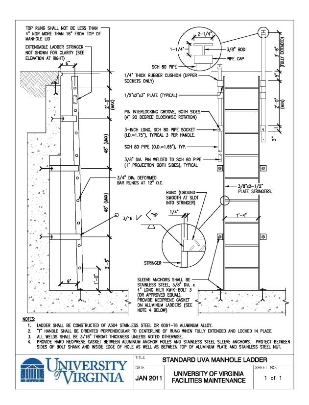
Figure 14: Standard UVA Manhole Ladder for Steam Tunnels and Manholes Greater than 10' Deep [not required for Electrical manholes]
