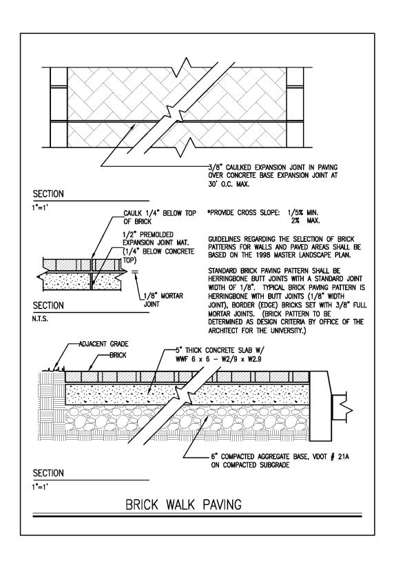
Figure 10: Brick Walk Paving
