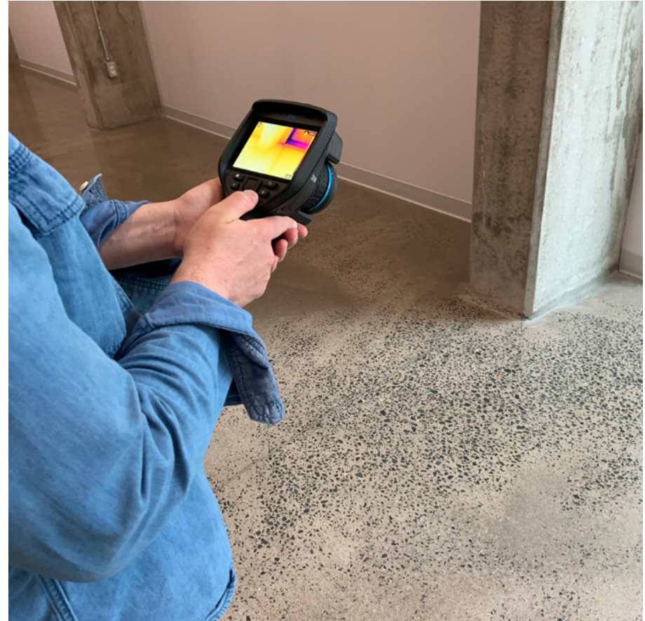
Photo 14. Air Leakage Testing at the IDEA Building
