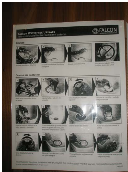
POSTED DIRECTIONS ON HOW TO CLEAN THE WATERLESS URINALS
