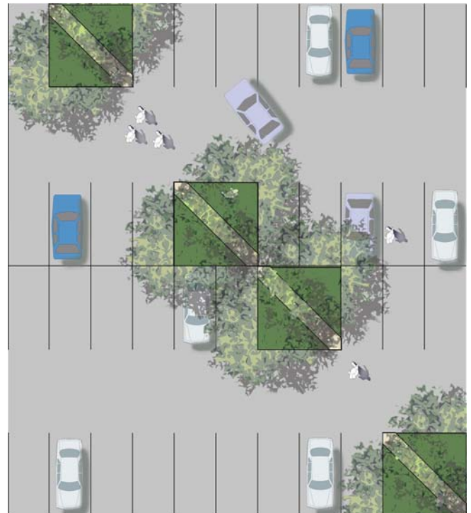
Biosquares are openings in the pavement at low points to capture storm water. They may be configured to allow pedestrian circulation across the parking lot in dry times.
