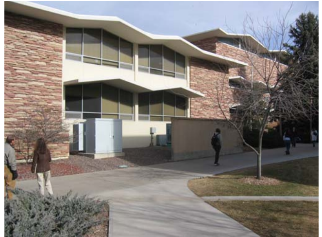
This on-site building equipment is not well screened from the public view.
