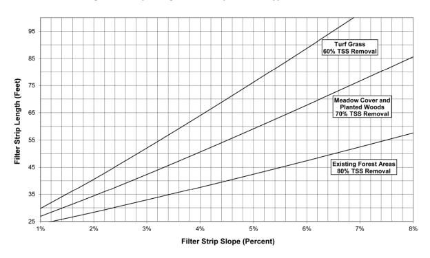
Drainage Area - Hydrologic Soil Group B & Soil Type = Loam, Silt Loam
