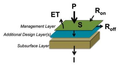
Figure 4.1: A conceptual diagram of the water balance of a unit.
