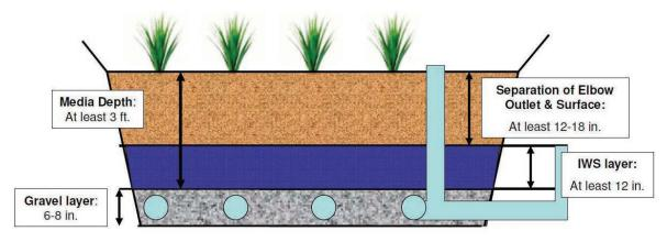
Figure 11: Bioretention cell showing IWS zones (Source: NCDENR).
