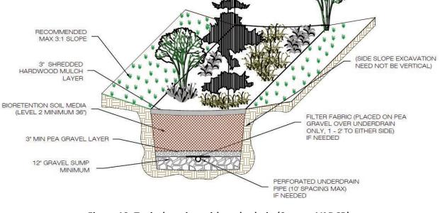
Figure 19: Typical section with underdrain (Source: VADCR).
