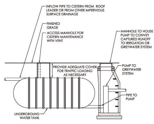
Figure 5: Cross-section of an underground cistern (Source: CHCRPC).
