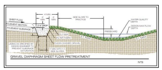
Figure 5: Pretreatment – gravel diaphragm for sheet from impervious or pervious surface (Source: West Virginia).
