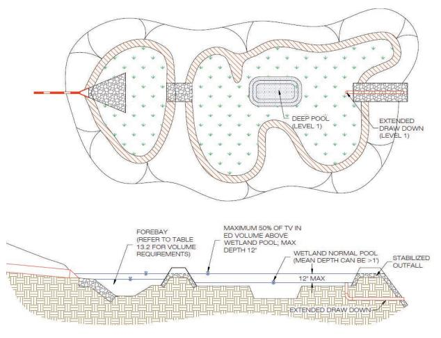
Figure 4: Constructed Wetland Plan and Cross Section.
