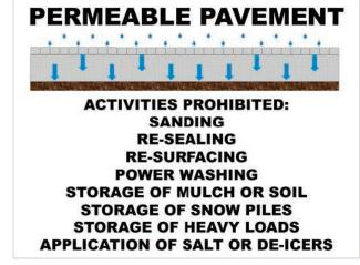
Figure 14: Example of permeable pavement signage (Source: NCDENR).
