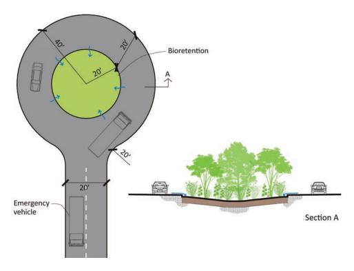
Figure 3.8: Cul-de-sac with bioretention.
