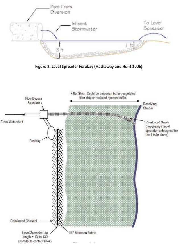
Figure 3a: Engineered Level Spreader (ELS) Plan (Hathaway 2006).
