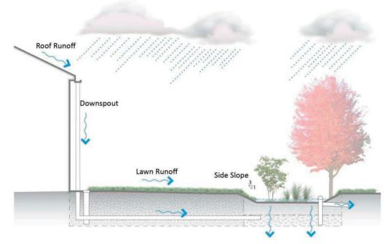
Figure 10: Roof leaders can convey high-velocity flows from the roof directly into the stone bed to prevent erosive conditions (Source: CHCRPC).
