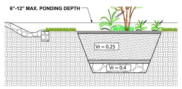
Figure 14: Typical bioretention section with void ratios for volume computations (Source: CHCRPC).
