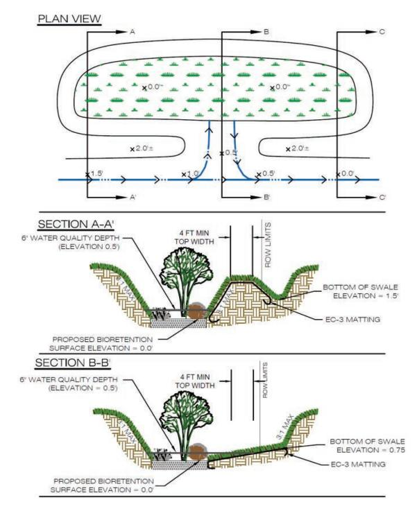
Figure 13: Typical Details for Off-Line Bioretention (Source: VADCR).
