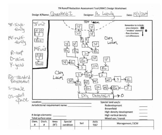
Figure 6.6: Design Worksheet from the common space management approach of a greenfield development in Knox County, TN.
