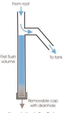
Figure 6: Simple first flush diverters (Source: Boodram and Cox).
