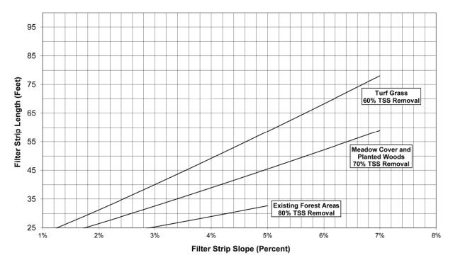
Figure 5: Graph may be used to estimate filter strip width based on soils, slope, and vegetation (Adapted from New Jersey Stormwater Management Practices Manual, Chapter 9, 2004).
