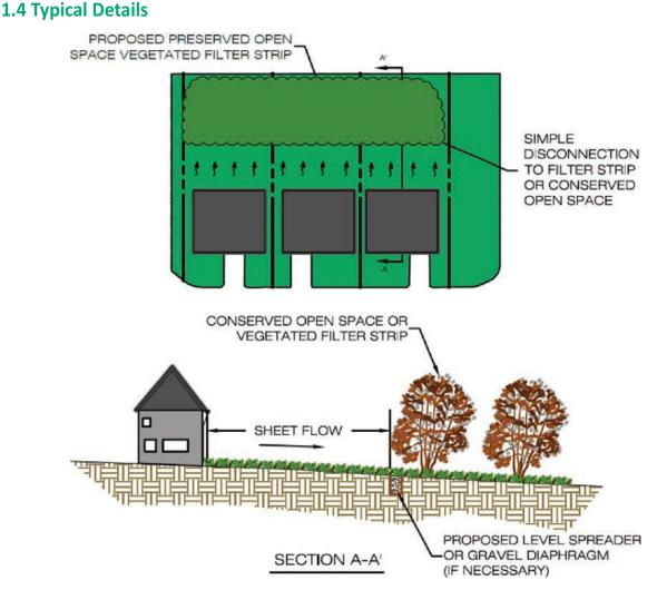
Figure 10: Simple disconnection to downstream preserved open space or vegetated filter strip (Source: Virginia, 2001).
