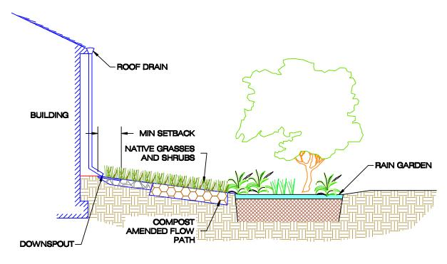
Figure 7: Rooftop Disconnection – Section View: Simple disconnection to downstream bioretention (Source: VADCR, 2011).
