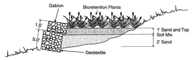
Figure 25: Bioretention suitable for use on slopes 10-20% (Source: NCDENR).
