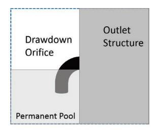
Figure 5.12: A drawdown orifice comprised of a downward turned elbow as part of an outlet structure to prevent clogging.
