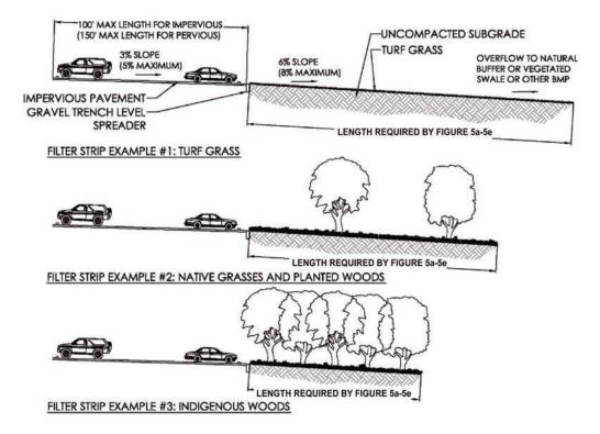
Figure 4: The width of a vegetative filter strip is determined by the slope, soil type, and vegetation type. For example, more densely vegetated strips are shorter in length than grass strips (Source: CHCRPC).
