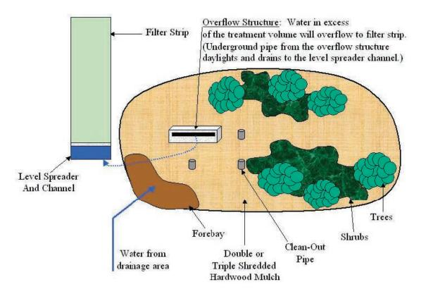
Figure 12: Bioretention units can be designed using an overflow device so that water in excess of the treatment volume overflows to a filter strip. This example shows a filter strip, though it is not required for every design (Source: NCDENR).
