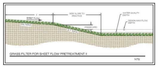
Figure 5: Pretreatment option – grass filter for sheet flow (Source: VADCR).
