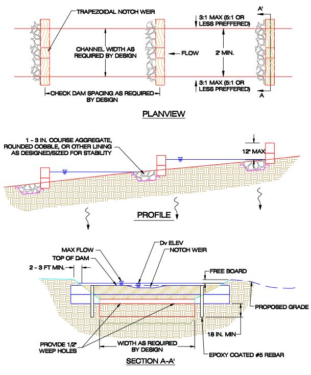
Figure 3: Grass swale with check dams – typical plan, profile, and section (Source: West Virginia).
