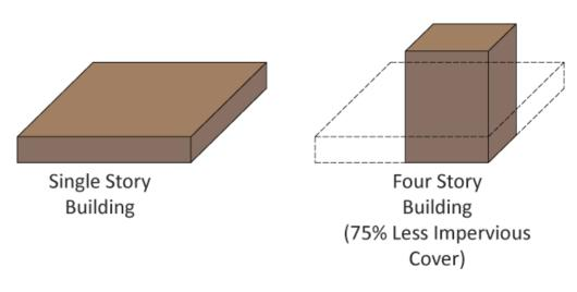
Figure 3.2: Simplistic representation of how a vertical design decreases the total amount of impervious surface created.
