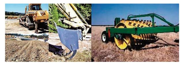
Figure 5.5: Attachments used for soil decompaction.
