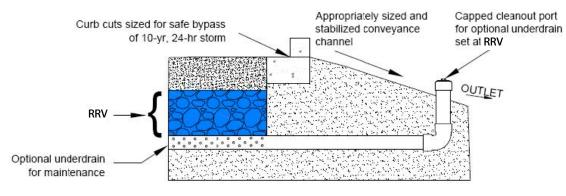
Figure 9: Bypass via curb cut and conveyance (PC only) (Source: NCSU-BAE).
