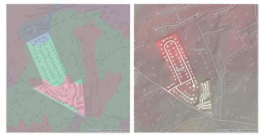
Figure 6.4: Project site maps with proposed plat overlay Left: Soil classifications (blue show silt loam, green and pink show clay loams) Right: Topographic map showing higher elevations on the north of the property (red) and lower elevations in the south end (tan).
