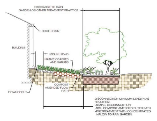
Figure 21: Residential Rooftop Disconnection to downstream raingarden – Bioretention without an underdrain (Source: VADCR).
