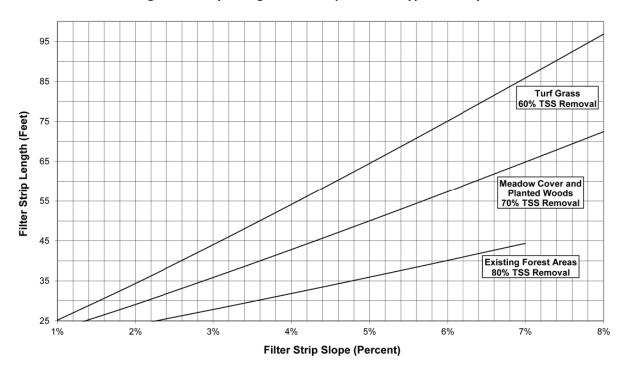
Drainage Area - Hydrologic Soil Group A & Soil Type = Sandy Loam
