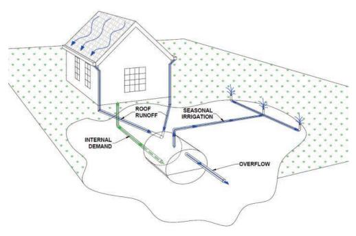
Figure 8. Configuration 1 Year-round indoor use with seasonal indoor and/or outdoor uses (Source: VADCR, 2013).
