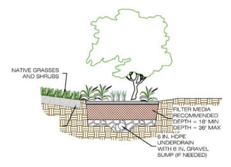
Figure 22: Bioretention with an underdrain (Source: VADCR).
