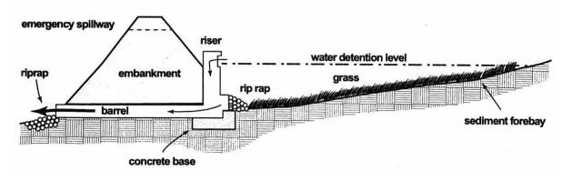
Figure 2: Dry detention pond cross-section (US EPA).
