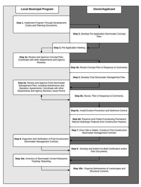
Figure 2.6: Typical Compliance Pathway for Permanent Stormwater Runoff Management for New Development and Redevelopment Projects. The following are recommended steps in Permanent Stormwater Management Control Implementation and Project-Level Compliance:
