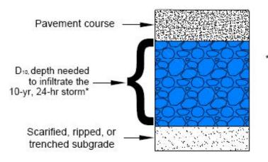
Note: See formula for D10 in this section. If RRV > D10, then set aggregate depth to RRV
