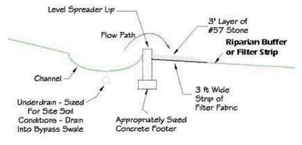
Figure 3b: Cross Section of Engineered Level Spreader (ELS) (Hathaway 2006).
