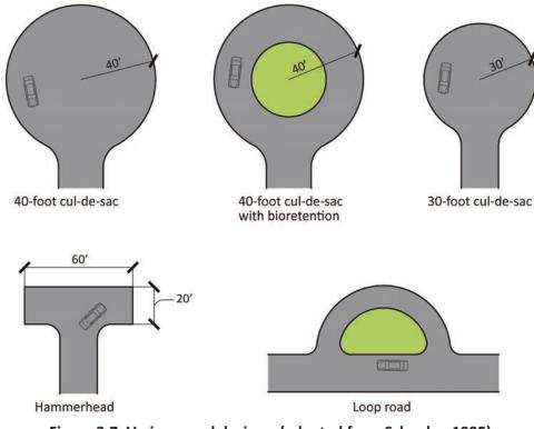
Figure 3.7: Various road designs. (adapted from Schueler, 1995).
