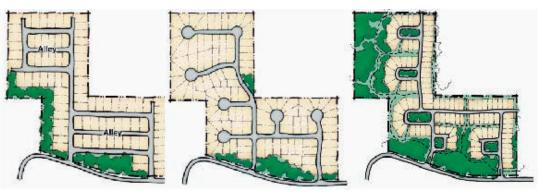
Figure 3.6: From left to right: grid, curvilinear, and hybrid pattern (AHBL Engineering).
