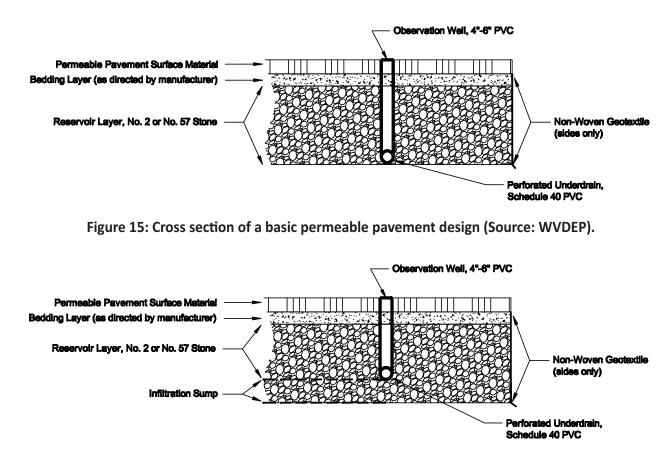
Figure 16: Cross section of a basic permeable pavement design with infiltration sump (Source: WVDEP).
