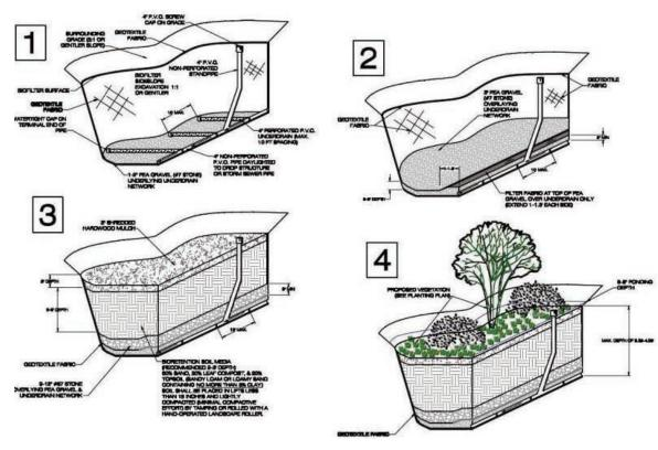
Figure 26: Typical bioretention construction sequence (Source:VADCR).
