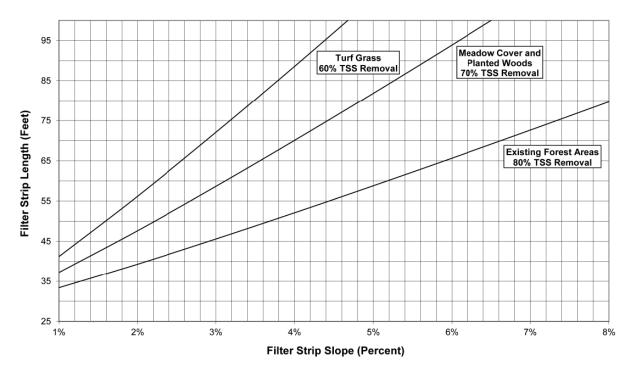
Drainage Area - Hydrologic Soil Group D & Soil Type = Clay Loam, Silty Clay, Clay
