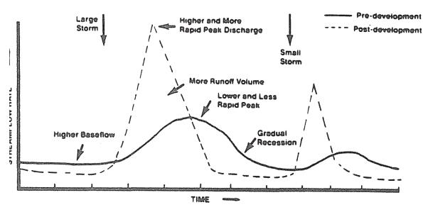
Figure 2.3: Changes in stream hydrology in response to development (From US EPA 2000 after Schuler, 1992).
