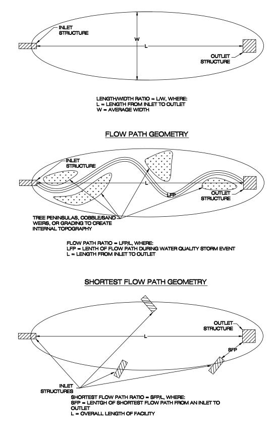
Figure 2: Design geometry factors: (1) Length/Width Ratio (top), (2) Flow Path Ratio (middle), and (3) Shortest Flow Path Ratio (Source: VA, 2011).
