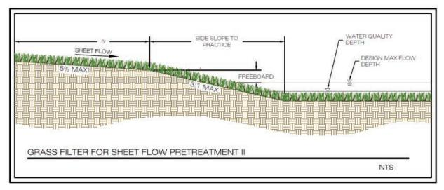
Figure 4: Pretreatment I and II – Grass filter for sheet flow (Source: West Virginia).
