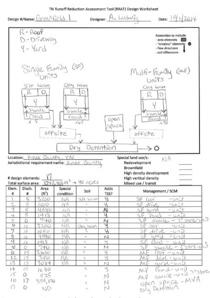
Figure 6.5: Design Worksheet from the lot-scale management approach of a greenfield development in Knox County, TN.
