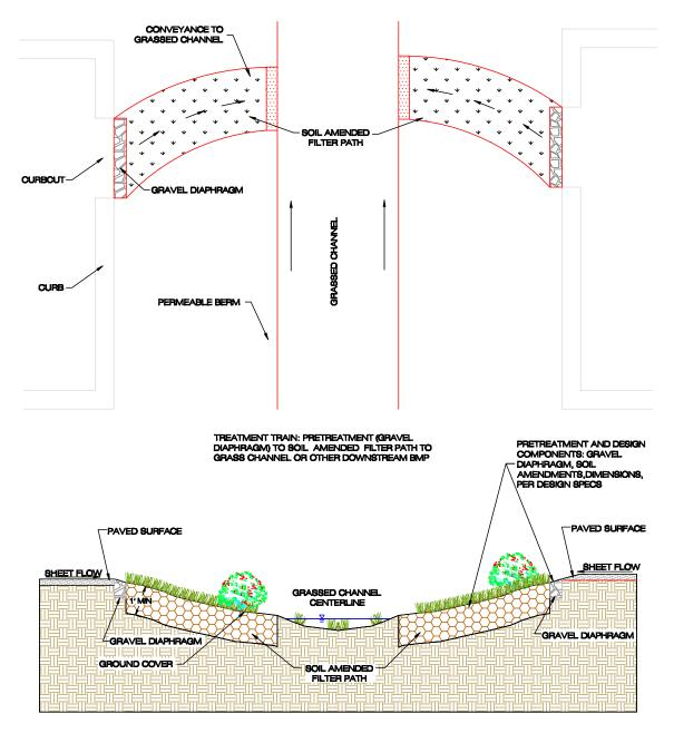
Figure 8: Filter path to grass channel (Source: Virginia).
