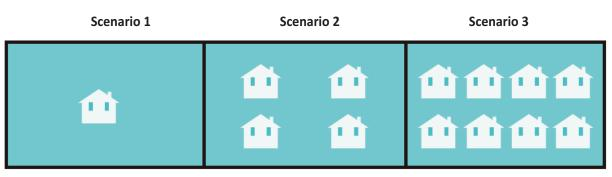
Impervious cover = 20% Runoff/acre = 18,700 ft<sup>3</sup>/yr Runoff/unit = 18,700 ft<sup>3</sup>/yr Impervious cover = **38%** Runoff/acre = **24,800** ft<sup>3</sup>/yr Runoff/unit = **6,200** ft<sup>3</sup>/yr Impervious cover = 65% Runoff/acre = 39,600 ft<sup>3</sup>/yr Runoff/unit = 4,950 ft<sup>3</sup>/yr
