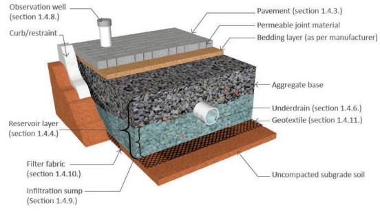
Figure 2: Schematic profile of permeable pavement.
