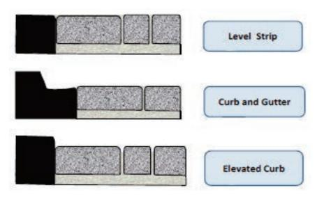
Figure 12: Examples of perimeter edge restraints (Source: NCDENR).
