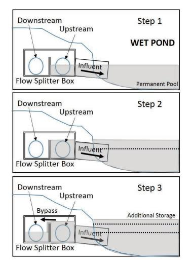
Figure 5.9: Water level progression in flow splitter box leading to a wet pond (Source: MCES, 2001).
