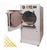
If your lab has an autoclave, routinely check for leaky valves and solenoid issues. A failed solenoid valve could waste 2.6 million gallons of water a year! Watch for signs of faulty valves. If you hear a gurgling sounds near the drain between cycles, the valve may be faulty. Report and replace any broken equipment.
