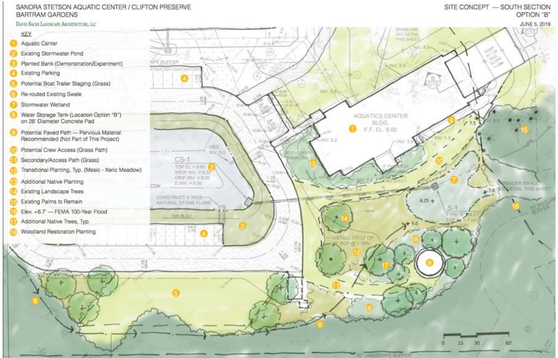
Figure 5: Alternative and Adopted Water Tank Siting with Rain Garden/Stormwater Wetland Design Sandra Stetson Aquatic Center
