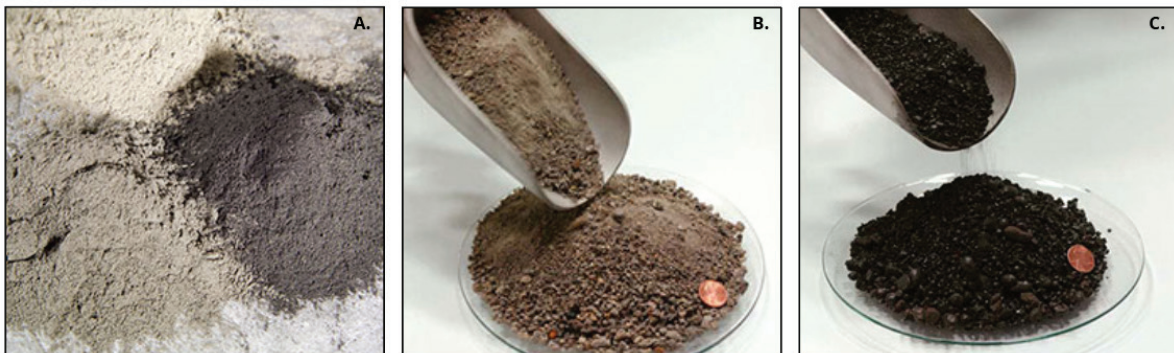
Types of coal ash: Fly ash (left), bottom ash (middle), and boiler slag (right). Credit: American Coal Ash Association
