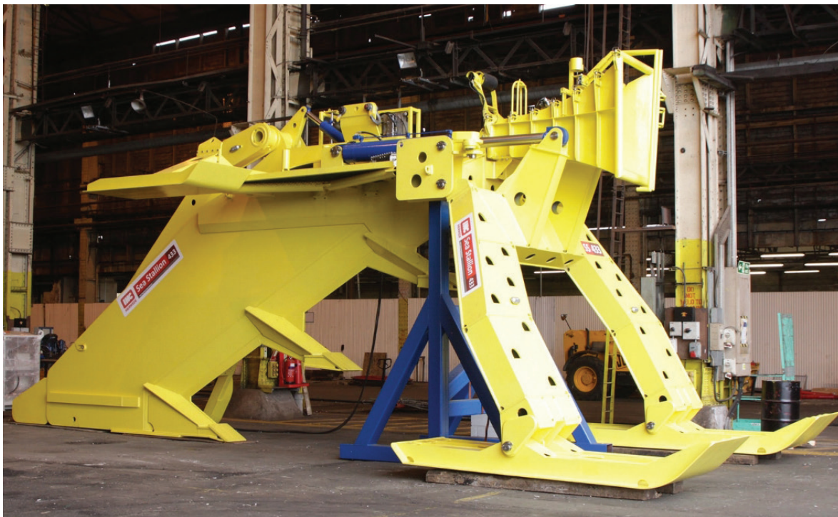
Manufactured by Royal IHC, this plow cuts the sea floor, making a trench for undersea cables. Credit: Royal IHC
