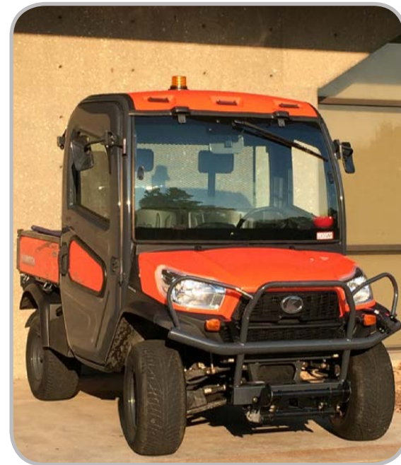
Figure 29: UNO has the opportunity to replace diesel utility vehicles like this one with electric options that cost less to operate, are quieter, and contribute less to outdoor air pollution.
