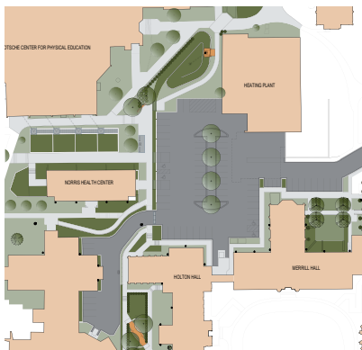
Lot 18- Pavilion Gateway Demonstration Project plan. In the demonstration project, the entire basin draining into Lot 18 is brought to the 100 year/ zero-discharge target. Lot 18 is expanded and reconfigured, while several other lots are eliminated or reduced. The bio-retention area is engineered to expand on the capacity assumptions of the masterplan.
