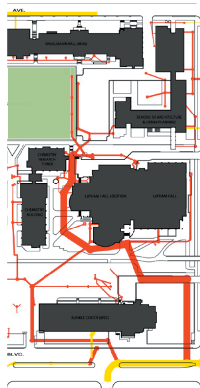
Storm Sewer Tree, Catchment 6. This storm sewer line drains Lapham Hall and the Chemistry buildings, with the Engleman Soccer field at the furthest extent. This is one of the largest trunk lines on campus, as indicated by the thickness of the red line. The yellow line at Kenwood Avenue is the combined storm and sanitary sewer of the City.
