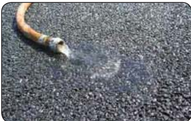
Fig. 4.14 Porous Asphalt Example (perviouspavement.org)
