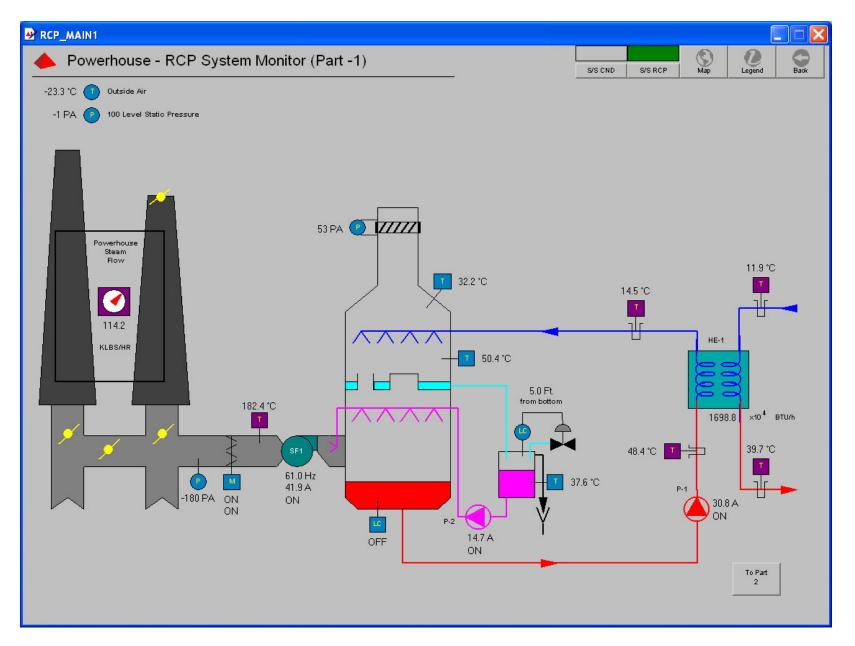
The recovery process is very simple. Water is sprayed into the flue gas. The flue gas cools as it warms the water spray. As the gas cools, water vapour in the gas (created by burning natural gas) begins to condense. The bulk of the recovered energy comes from the energy released from the water phase change, from vapour to liquid.
