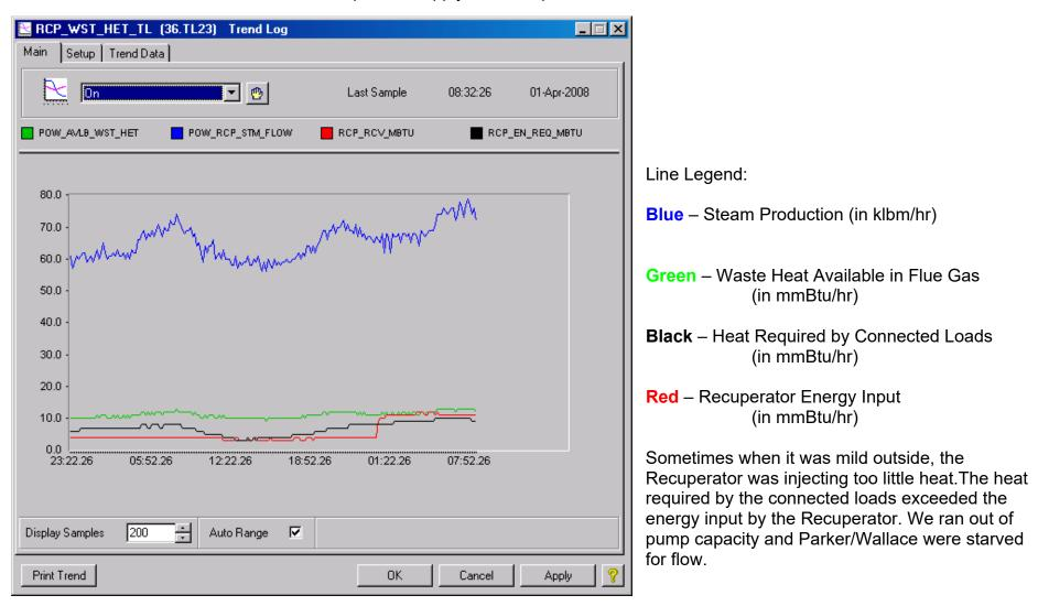
Sometimes when it was colder outside, the Recuperator injected too much heat. The Recuperator injected more heat than the connected loads required. The water-cooled condensers overheated because the minimum flow required at Animal Science returned water that was too warm.
