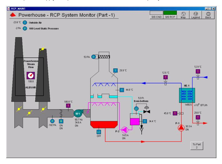
When it was cold outside and the Recuperator was running flat out, the 50 hp supply fan motor was only drawing 34.6 Amps.
