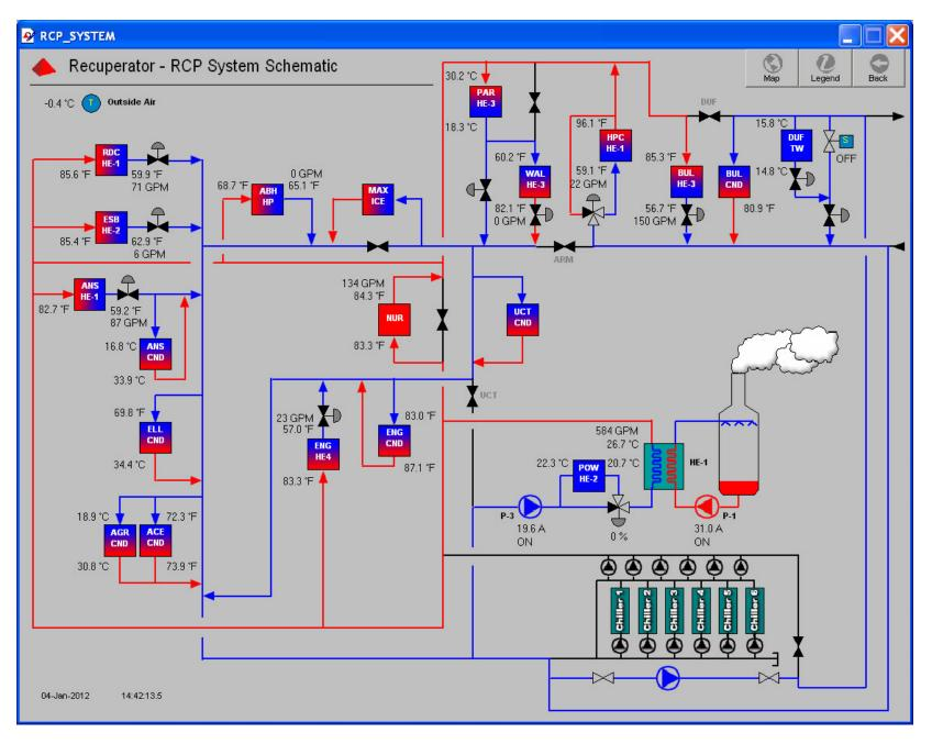
Most of the heat is used to preheat outside air. In laboratories, considerable make-up is required to offset the air exhausted by fumehoods. Connected load capacities greatly exceed the waste heat available.
