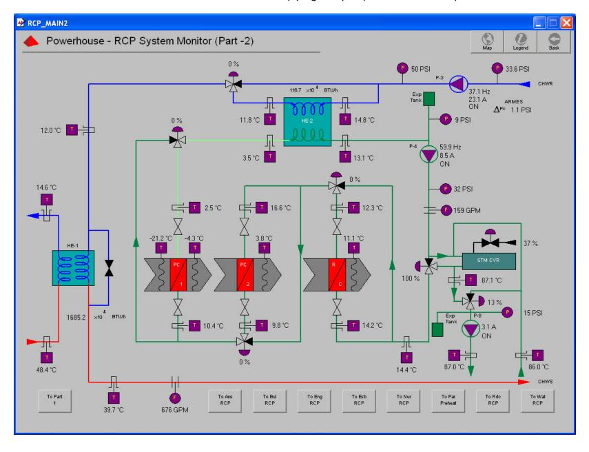
Additional heat is recovered from numerous water-cooled condensers scattered throughout the campus. Total combined capacity is 1.5 mmBtu/h.
