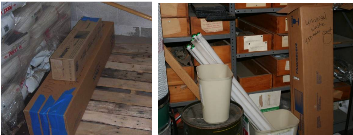
Figure 5.3. Campus examples of good universal waste handling practices (left) and practices needing improvement (right). Source: Victoria Justus, Turning Bird Consulting.
