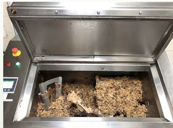
Figure 3B: Internal View (digesting "stomach") of the Digester
