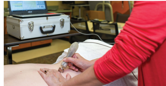
A force-sensing instrument for use during manual therapy
