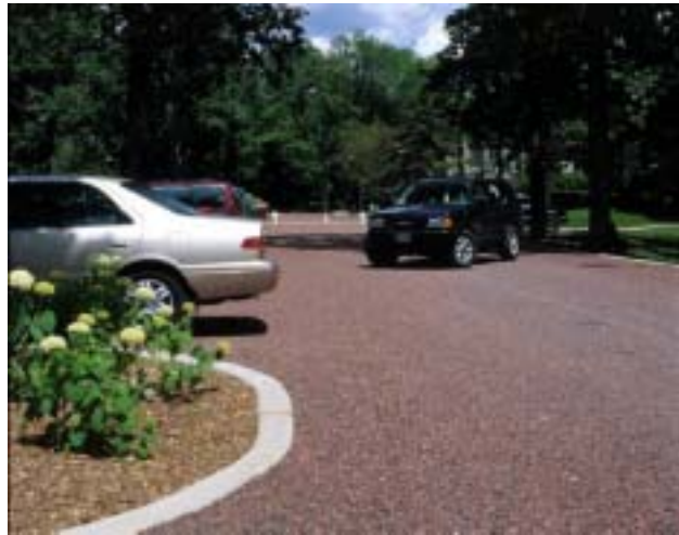
Minimizing impervious surfaces maximizes the area available for soils and vegetation to receive and treat surface water. NREL/PIX 11414
