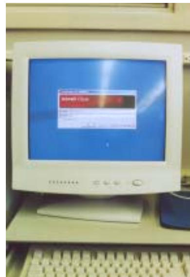
Reflections of luminaires in computer screens can cause veiling glare. Careful lighting and daylighting design avoids these problems.
